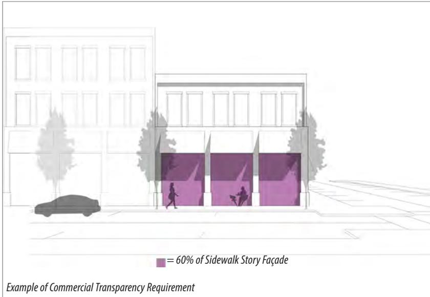
3. **Materials:** Building façade materials, with the exception of corner treatments and columns, shall be combined only horizontally, with the heavier below the lighter. The exterior finish material on all Façades shall be limited to brick, stone, and/or hard coat stucco.
